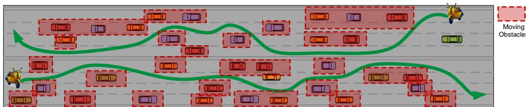
Figure 2 two-wheel vehicular macroscopic flow concept, where vehicles are considered as mobile obstacles to a fluid
